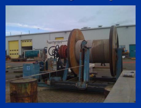
The drum is mounted on stub shafts either end with movable centres
